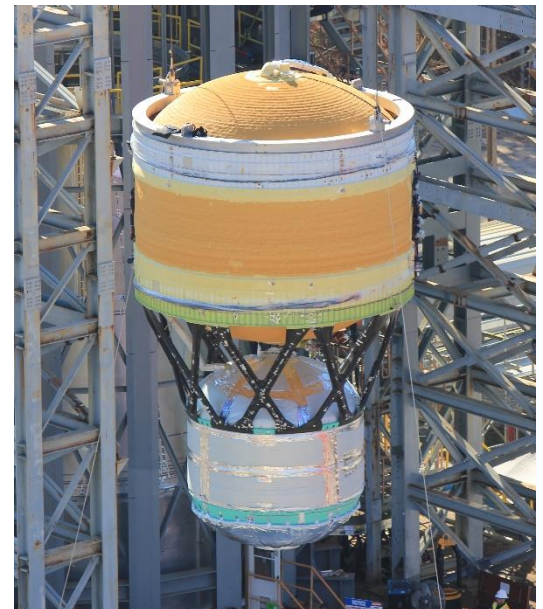
The Space Launch System's Interim Cryogenic Propulsion Stage will use liquid hydrogen and liquid oxygen to give the Orion spacecraft the in-space push needed to fly beyond the moon. Image Credit: NASA/MSFC/Brian C. Massey
